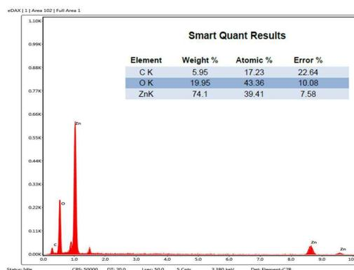
**Figure 3:** EDAX image displaying zinc and oxygen peaks, as well as their respective percentages
