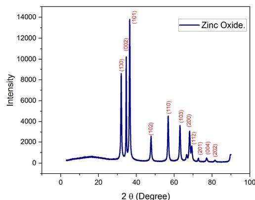
**Figure 4:** XRD of green synthesized Zinc Oxide nanoparticles
