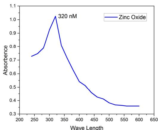
**Figure 1:** UV spectra of Green synthesized Zinc Oxide Nanoparticles ( $\lambda$  max at 320 nm)
