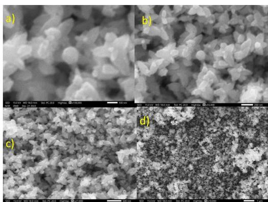
**Figure 2:** Green synthesised nanoparticles SEM images at various magnifications 100 nm, 200 nm, 500 nm, and 1 $\mu$ m is the range
