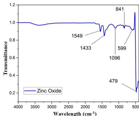
**Figure 5:** FT-IR analysis of green synthesised ZnO NPs
