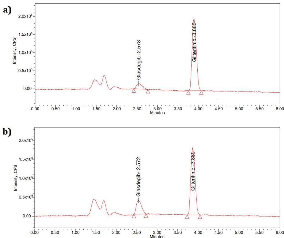
**Figure 8:** Chromatogram of (A) LOD & (B) LOQ
