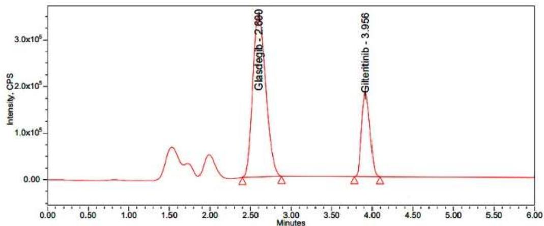
**Figure 2:** Chromatogram for System Suitability
