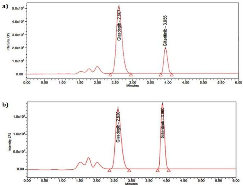
**Figure 5:** Matrix Effect of Chromatograms (A) HQC & (B) LQC
